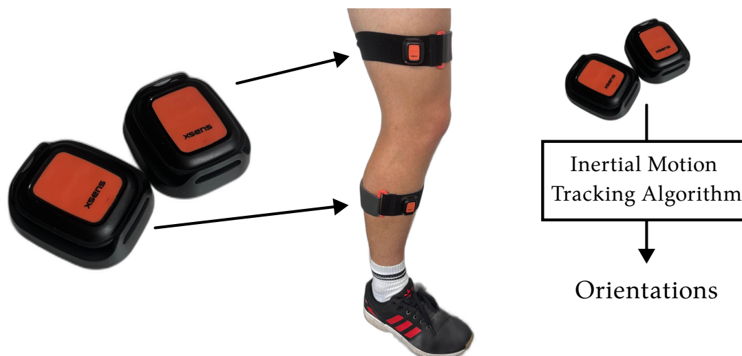
Figure 1.7: Two IMUs (Inertial Measurement Units), Xsens Movella Dots, are attached to the upper and lower leg, and IMT (Inertial Motion Tracking) algorithms can be used to track its motion. IMT algorithms use sensor fusion to combine IMU measurements, consisting of 3D (Three-Dimensional) accelerometer, 3D gyroscope, and 3D magnetometer, and estimate a trajectory of orientations.
