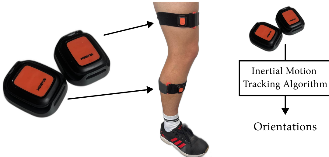
Figure 1.7: Two IMUs (Inertial Measurement Units), Xsens Movella Dots, are attached to the upper and lower leg, and IMT algorithms can be used to track its motion. IMT algorithms use sensor fusion to combine IMU data (3D (Three-Dimensional) accelerometer, 3D gyroscope, 3D magnetometer) and estimate a trajectory of orientations.
