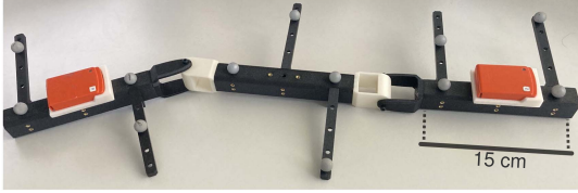
Fig. 2. 3D-printed kinematic chain used for recording experimental data. Three segments (black) connected by two hinge joints (white) with nonparallel joint axes. A sparse set of two IMUs (orange) are attached to the outer segments. Gray spheres are OMC markers.
